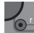
-20°C至+60°C时，最 小弯曲半径6D -30°C至-20°C r=6D for temperature from -20°C to +60°C r=12D for temperature from -30°C to -20°C
